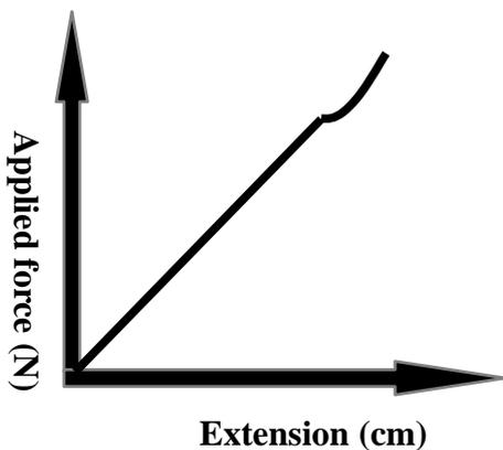
Plotting an extension against the force applied produces a straight line until the spring is stretched beyond its **elastic limit**, as shown in the figure. The elastic limit is the point at which the force applied is too great for the spring and it no longer returns to its original length when the force is removed.
