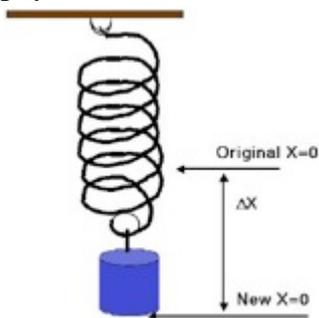
We can see Hooke's law in action when masses are hung on the end of a spring, as in the figure. Each 100g of mass hung on the spring will apply a force of 1,0N that stretches the spring. Each time an extra 1,0N force is applied, the length of the spring will increase by the same amount. The length of the spring without any force applied to it is called the **original length**. The total increase in length of the spring is called the **extension**.
